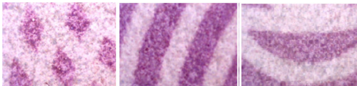
Figure 2. Non-irradiated (light) and irradiated (dark) areas in SPLC films (60×).
