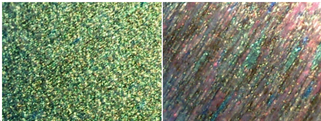
Figure 7. Stretched SPLC polymer films with microcapsules.
