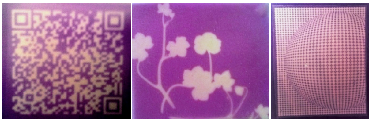
Figure 10. Optical recording images with high contrast by UV light in SPLC polymer films.
